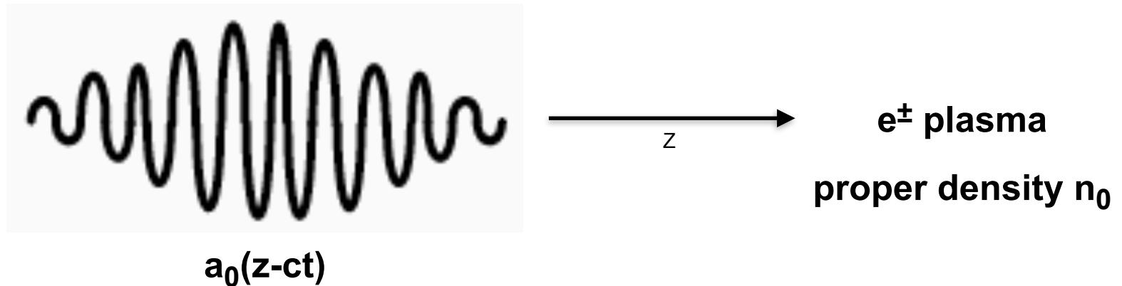
$$\frac{\text{particles kinetic energy}}{\text{wave energy}} = \left( \frac{a_0 \omega_P}{\omega} \right)^2$$
